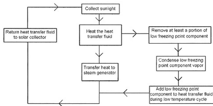
*The heat transfer system involves a variable composition heat transfer fluid. The low freezing point component of the heat transfer fluid is removed and re-added.*
