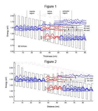
The active region of the semiconductor structures of this invention includes upper energy states 4, 5 and 6, where the energy difference between energy states 4 and 5 is denoted by E54 and the energy difference between energy states 5 and 6 is denoted by E65. The semiconductor structures of this invention (Figure 2) provide much greater values of E54 and E65 than conventional QCL structures (Figure 1), resulting in virtually complete suppression of electron leakage
