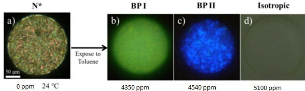
Sample phase and color changes for blue-phase liquid crystals at different toluene concentrations
