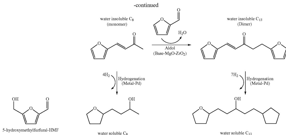
Reaction Scheme 6 shows the corresponding set of reactions wherein furfural and acetone are the reactants for the initial aldol condensation reaction (rather than hydroxymethylfurfural or hydroxymethyltetrahydrofurfural, as shown in Reaction Scheme 5).
