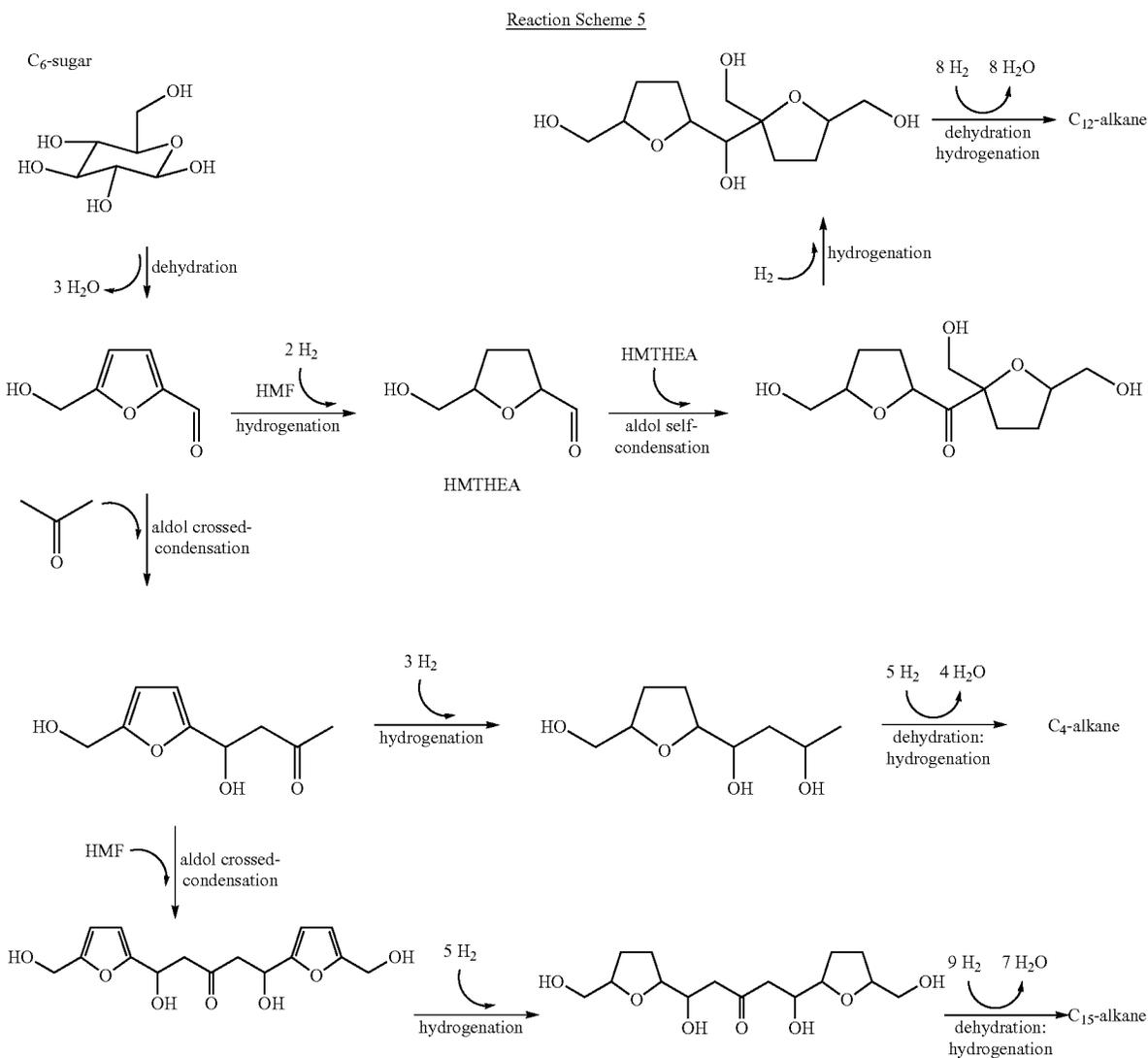
Crossed aldol condensation of HMF with acetone was carried out with HMF:acetone molar ratios of 1:1 and 1:10 using a mixed Mg—Al-oxide catalyst at room temperature (see Tables 4 and 5, entries 6 to 9). The Mg—Al-oxide catalyst was prepared by co-precipitation, similar to the method reported elsewhere. Sasaki, Goto, Tajima, Adschiri & Arai (2002) *Green Chem.* 4:285. Climent, Corma, Iborra, Epping, & Velty (2004) *J. Catal.* 225:316.
