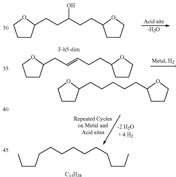
If the feed to this final step is not fully hydrogenated (i.e., if the effluent from the hydrogenation is not solely in the F-h4-mon and F-h5-dim forms), the metal in this step will hydrogenate these species. However, if the feed contains too many double bonds, the final step cannot be accomplished with high yields due to the formation of undesirable carbonaceous deposits on the catalyst.
