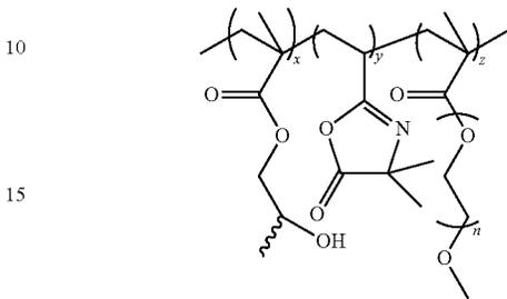
wherein x, y and z represent the mole fractions of the crosslinked monomer, the 4,4-dimethyl-2-vinylazlactone monomer and the polyethylene glycol methyl ether methacrylate monomer; n represents the number of repeat units in
