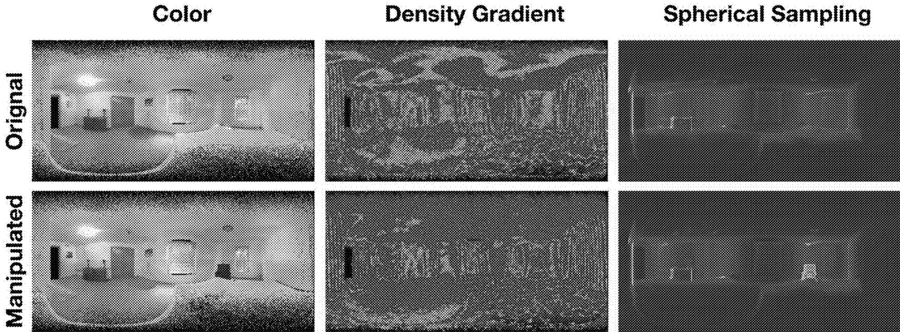
Down-sampled Point Cloud Before and After a Manipulation to add a Chair to the Scene with Density Gradient and Spherical Sampling Visualized
