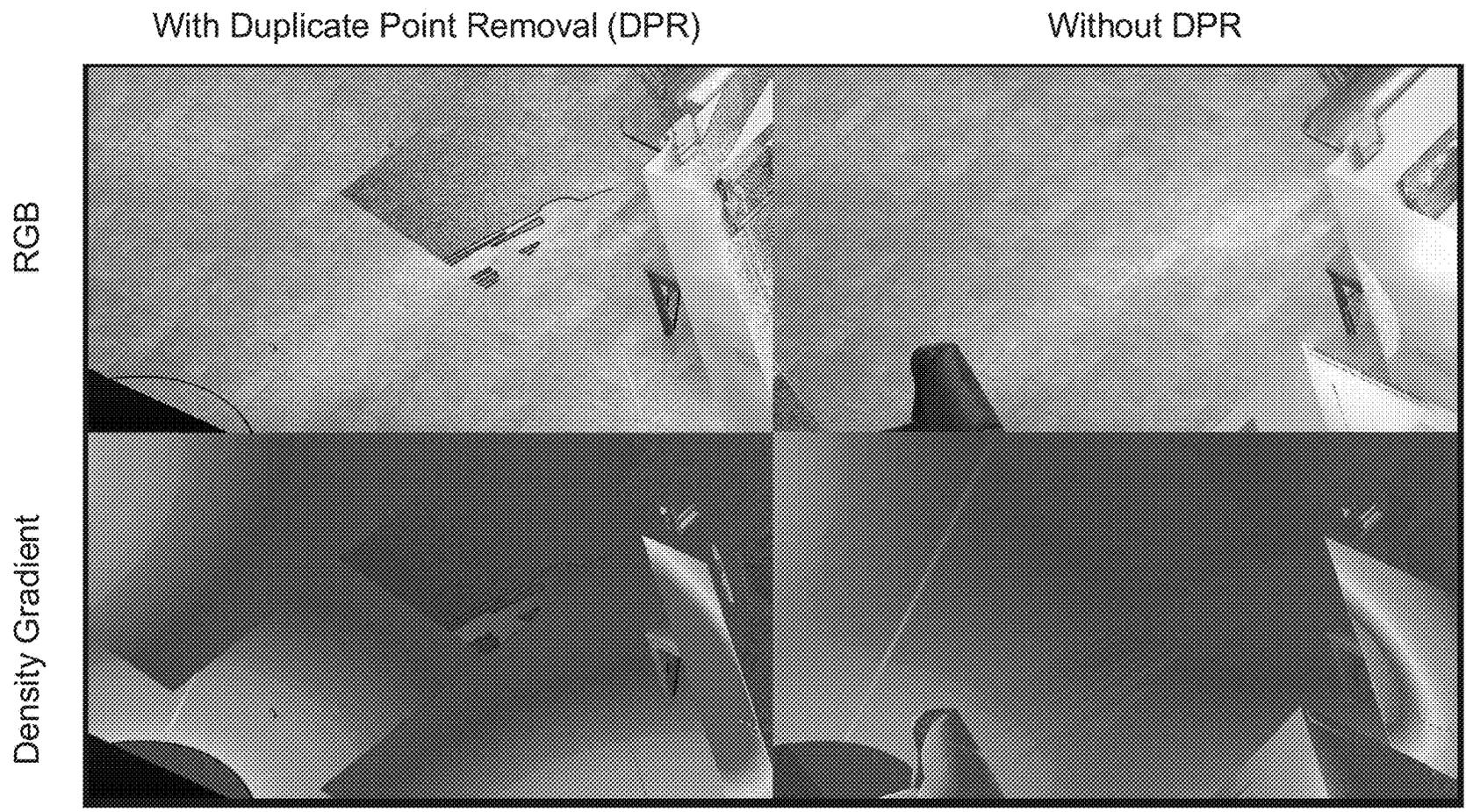
Point Clouds of a Scene Combined with and without Duplicate Point Removal and Representations Based on Density of Points by Location in Scene
