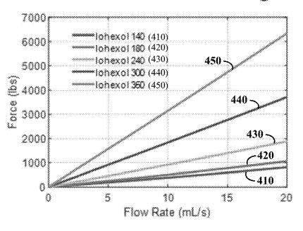
Actuator Pressure vs Commanded Flow Rate @ 20 °C
