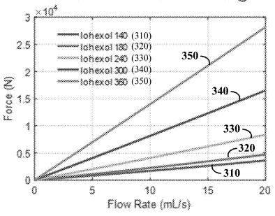
Actuator Force vs Commanded Flow Rate @ 20 °C
